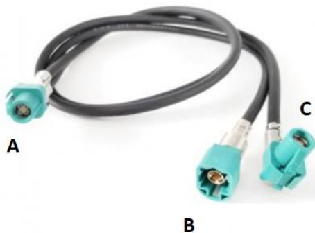
**Plug A** has a double cable, it must be on the interface. Stightens **plug B** of the video cable on the counter-plug of the video cable from the multimedia unit.
