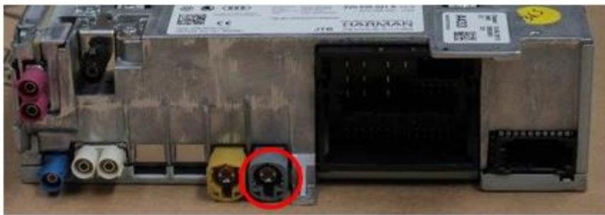
Press the grey or pink video connector into the pallet at the bottom. Pry very carefully with a small flat object between the seam if the plug is very tight. Leave the rest of the plugs plugged in. If necessary, cut some tape between the cables so that there is enough freedom of movement to pull the thick cable and the video cable out of the housing.
