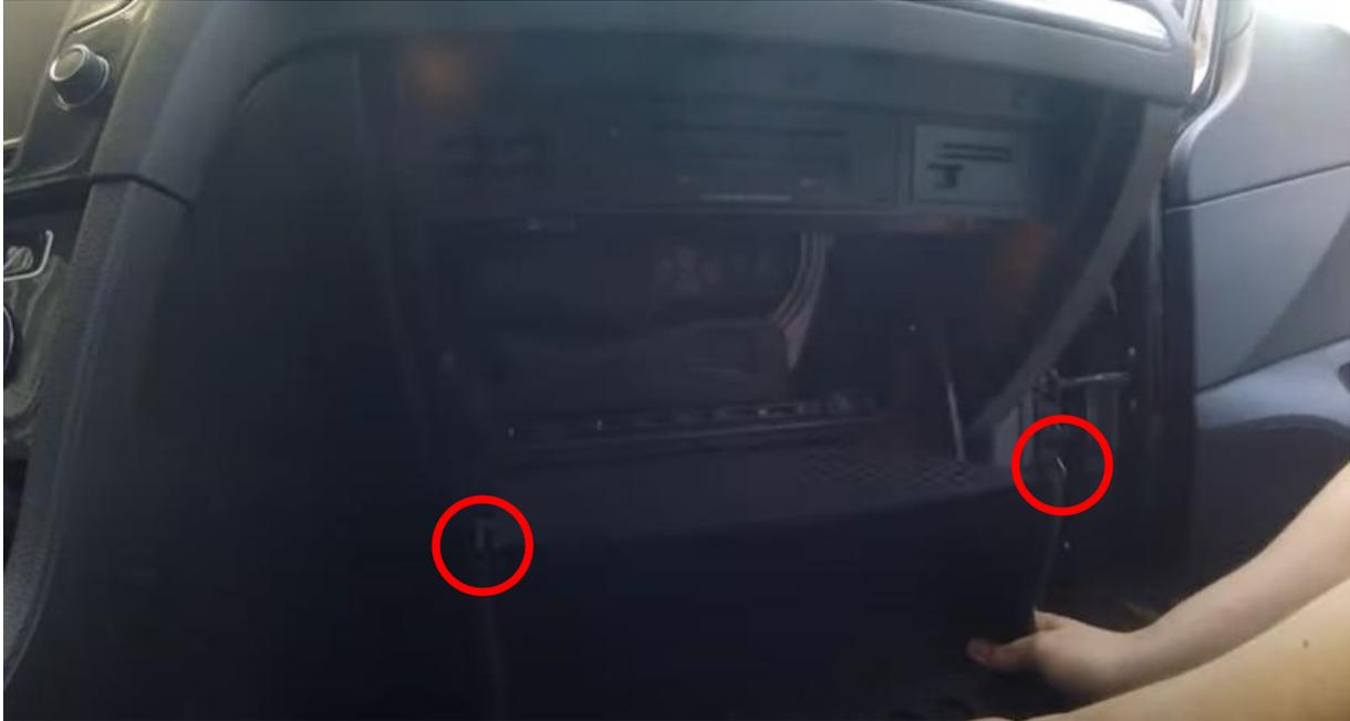
If this simple method is not possible Google then on "remove glovebox VW", there are multiple videos on the internet how to remove the glove box. In most cases, it is a matter of unscrewing the glove compartment in its entirety at the top and bottom. Remove the cover under the air conditioning unit to unscrew 1 additional screw. This screw prevents you from removing the glove compartment. Removing the cover may be sufficient. If not, you need to click away some extra panels all around.
